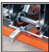
Detach device for heater
