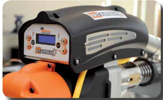
K-SB 40 is a compact and ergonomic extruder equipped with a power control device and the safety system “motor block” that doesn’t allow the machine to start before it reaches the right temperature. The extruder has an innovative universal feeding system that makes possible to use the machine with different diameters of wire.
