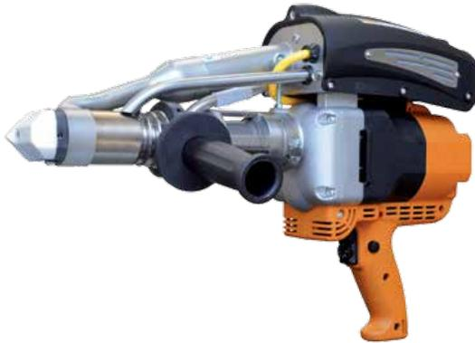
K-SB 20 is a compact and ergonomic extruder equipped with a power control device and the safety system “motor block” that doesn’t allow the machine to start before it reaches the right temperature. The extruder has an innovative universal feeding system that makes possible to use the machine with different diameters of wire.
