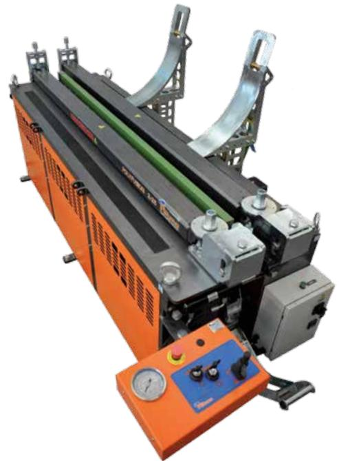
POLYFUSION 2-25 and POLYFUSION 2-50 are compact and easy to use manual welders for HDPE and PP sheets from two meters wide and 3÷25 mm or 1/8"÷1" thickness (mod. POLYFUSION 2-25); and 3÷50 mm or 1/8"÷2" thickness (mod. POLYFUSION 2-50). The machines can also weld twin-wall sheets. The machine can operate in compliance with the D.V.S. 2207.
