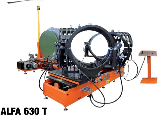
Workshop welding machine designed to fabricate fittings like elbows, wyes, tees and crosses (up to  $\emptyset$  630 mm or 24" DIPS). All jaws movements are electro-hydraulically operated, both the open/close movement and the blocking mechanism.
