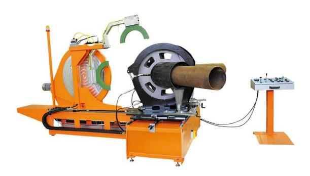
ALFA TEL - 800 is a workshop machine designed to weld pre-insulated district HDPE pipes and valves for both heating and cooling lines.
